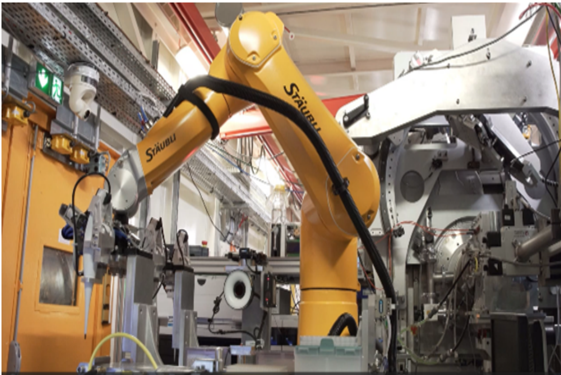
Figure 2: Robotic Arm installed on the SWING beamline.
